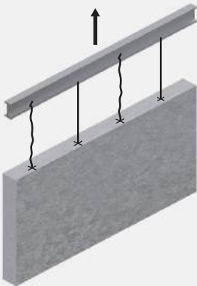
Assume 2 anchors take the load
