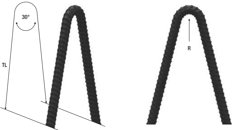
TL = Total length of rebar, before bending
