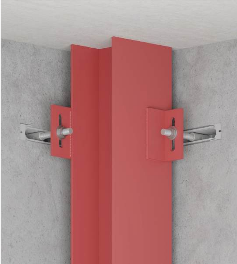
Panel to Steel Column Connection
